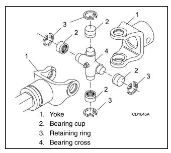
Figure 22. U-Joint Exploded View
